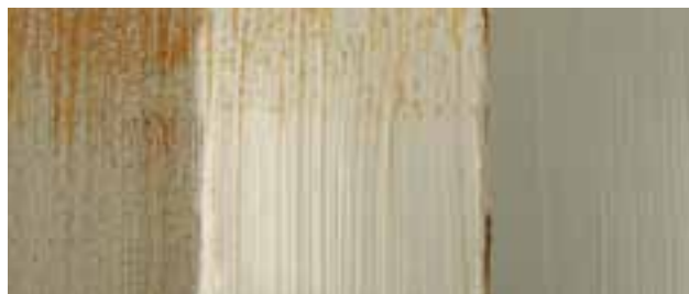
Typical brush application of traditional epoxy mastic coatings (left & centre) and Jotamastic Smart Pack (right) after continuous exposure in a salt water chamber.
